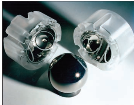
One of the four gyroscopes – a perfect niobium-coated quartz ball – and its housing equipped with six electrodes to suspend the ball electrically, and a channel to spin it up with a stream of helium. (Image credit: Gravity Probe B.)
