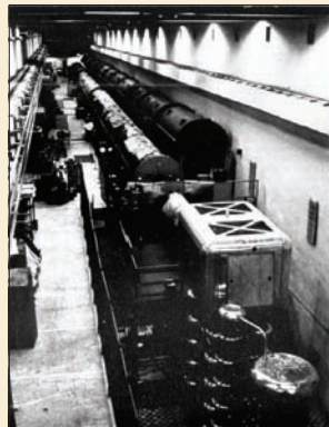
The Serpukhov linear accelerator/injector with the vacuum lids removed. (Image credit: Serpukhov.)
